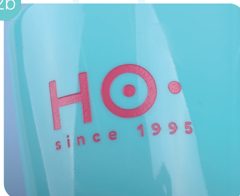
Outer coloring and logo sandblasting (deep engraving) with color fill
